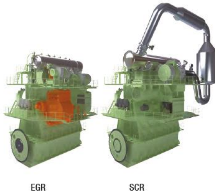
Fig. 1.02: Two-way approach for Tier III engine – EGR and SCR solutions
